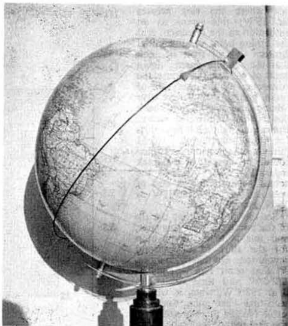
The globe used by the writer for plotting orbits. The ring is set to the inclination angle of the satellite.
