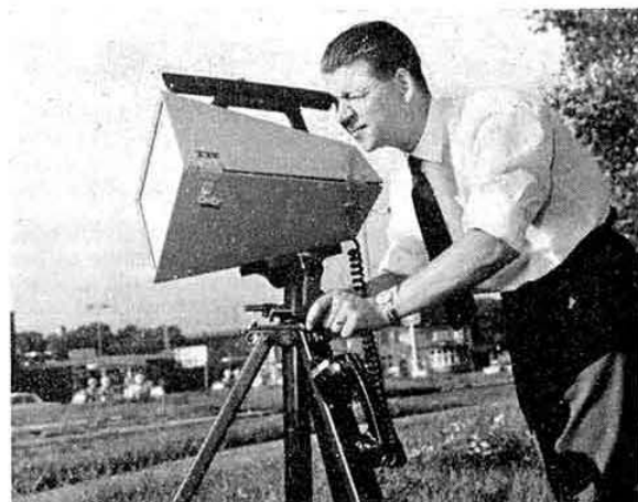
An experimental microwave communications terminal using thick-film micro-electronics and weighing 17 lb. Varactor multipliers provide some 200 milliwatts at 4500 Mc/s. The equipment was developed by IIT Federal Laboratories and demonstrated in the UK by the associated company STC.
